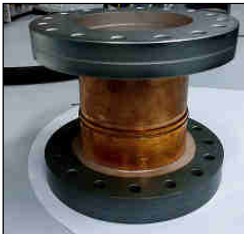
Fig.7: Developed single disc alumina RF window
