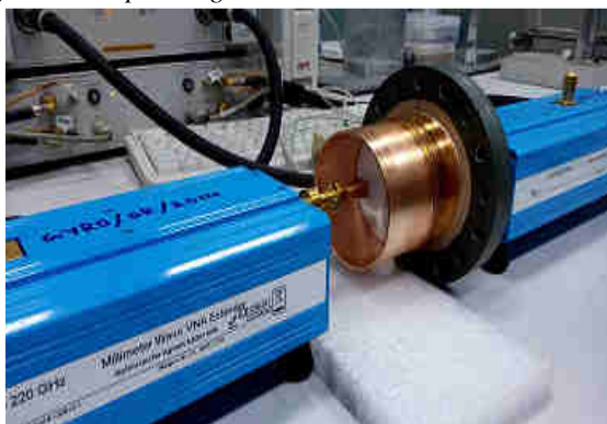
Fig.8: Cold test setup of RF window using free space method
